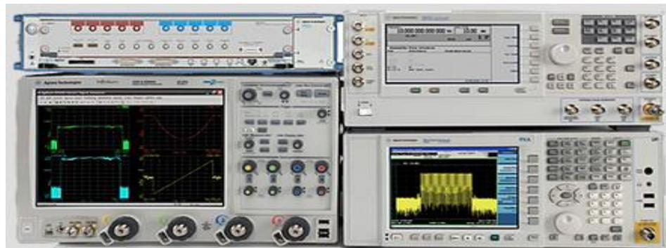
Figure 1: This four-instrument test setup enables testing of both receivers and transmitters.
